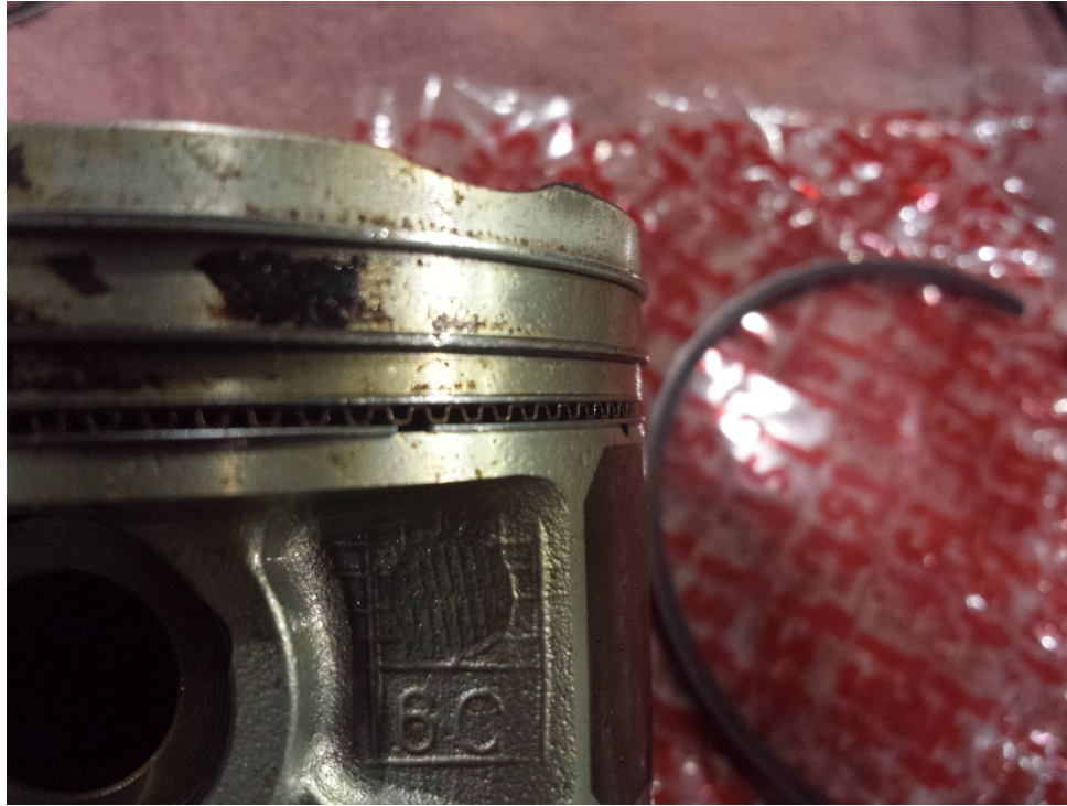
FB20 Piston with Worn Oil Control Ring
