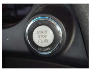
10. The Keyless Fob never needs to come into physical contact with the vehicle in order to start the engine. Instead, a Keyless Fob can remain in the driver's pocket, purse, jacket, or even on the passenger seat or elsewhere in the car and still be used in conjunction with the start/stop button to start the engine.
