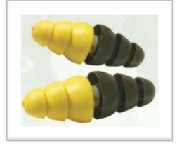
could be inserted into the ear canal. The olive end was closed and meant to block all sound like a traditional earplug. The yellow end was open, to a small extent, to allow the wearer to hear certain sounds, such as spoken commands, while still offering protection from damaging impulse sounds.
