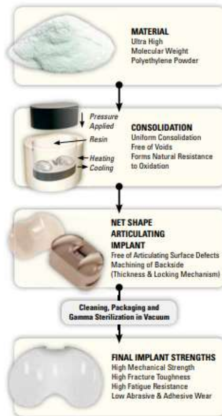
FIGURE 12: Manufacturing Process for NCM Polyethylene Inserts
