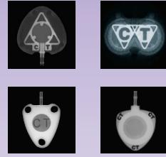
Radiopaque identifiers for PowerPort® devices aid in identification as a Bard power injectable port.
