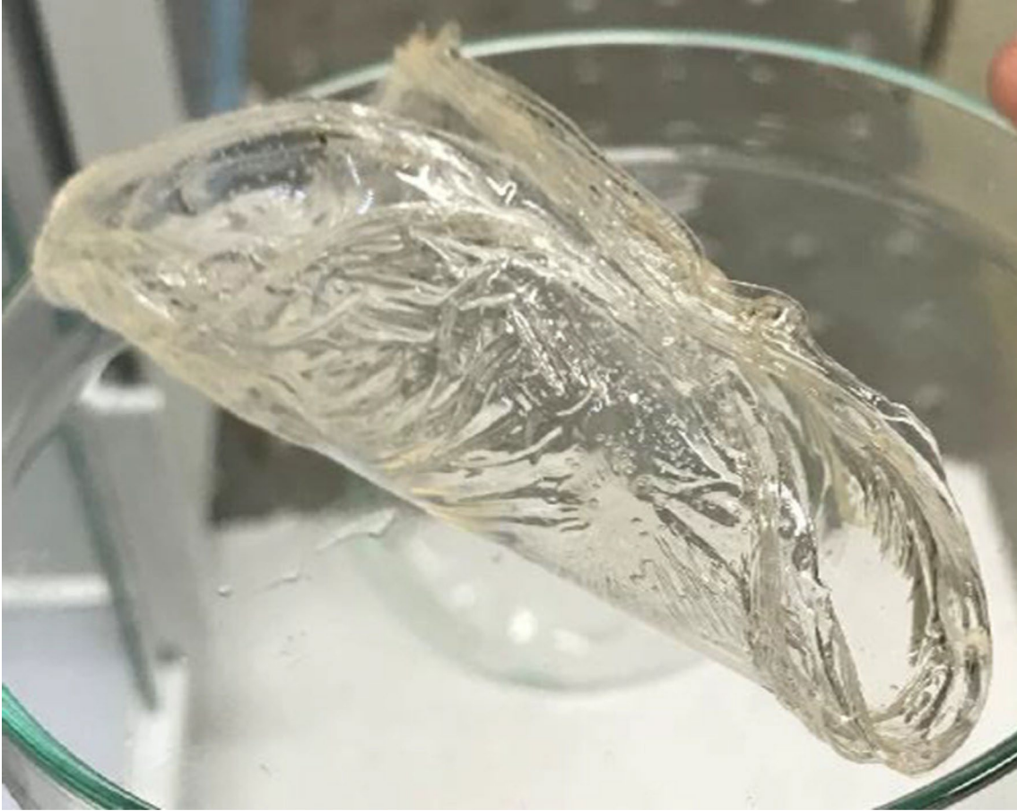
Figure 4 - Semi-irreversible contracture of thick PVA hydrogel
