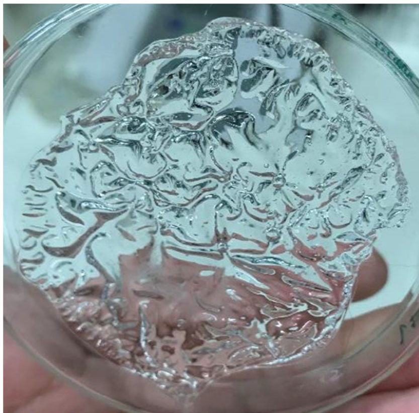
Figure 2 - Striations on gel caused by rapid cooling and oxygenation of pre gel solution.
