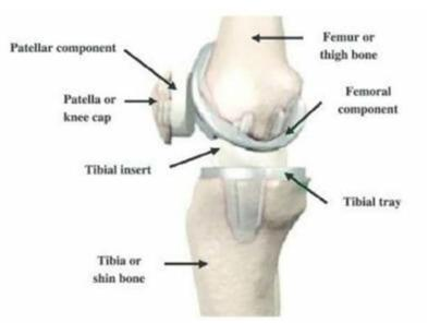
32. The patellar cap and tibial insert are made of polyethylene.
