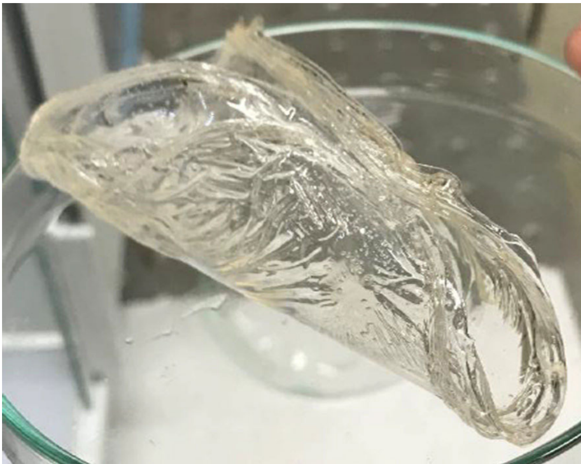
Figure 4 - Semi-irreversible contracture of thick PVA hydrogel
