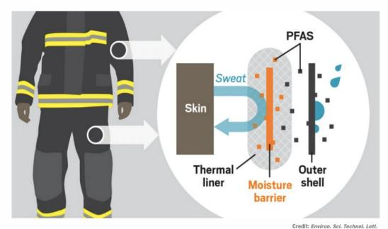
Over time, PFAS in a firefighter's turnout gear can migrate from a moisture barrier (orange) into a thermal liner that contacts skin. PFAS can also be shed from an outer shell (black) into the environment.
