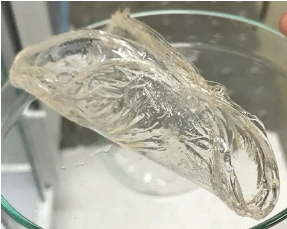
Figure 4 - Semi-irreversible contracture of thick PVA hydrogel
